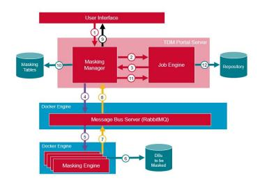
5 Masking engine pulls task from queue, each docker container contains four masking engines
