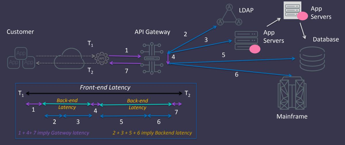
Customer use app which calls an API on a gateway (front-end). APIs policies call different back-ends including LDAP, app server, database, mainframe and etc. Now we can pinpoint the customer's transaction latency!
