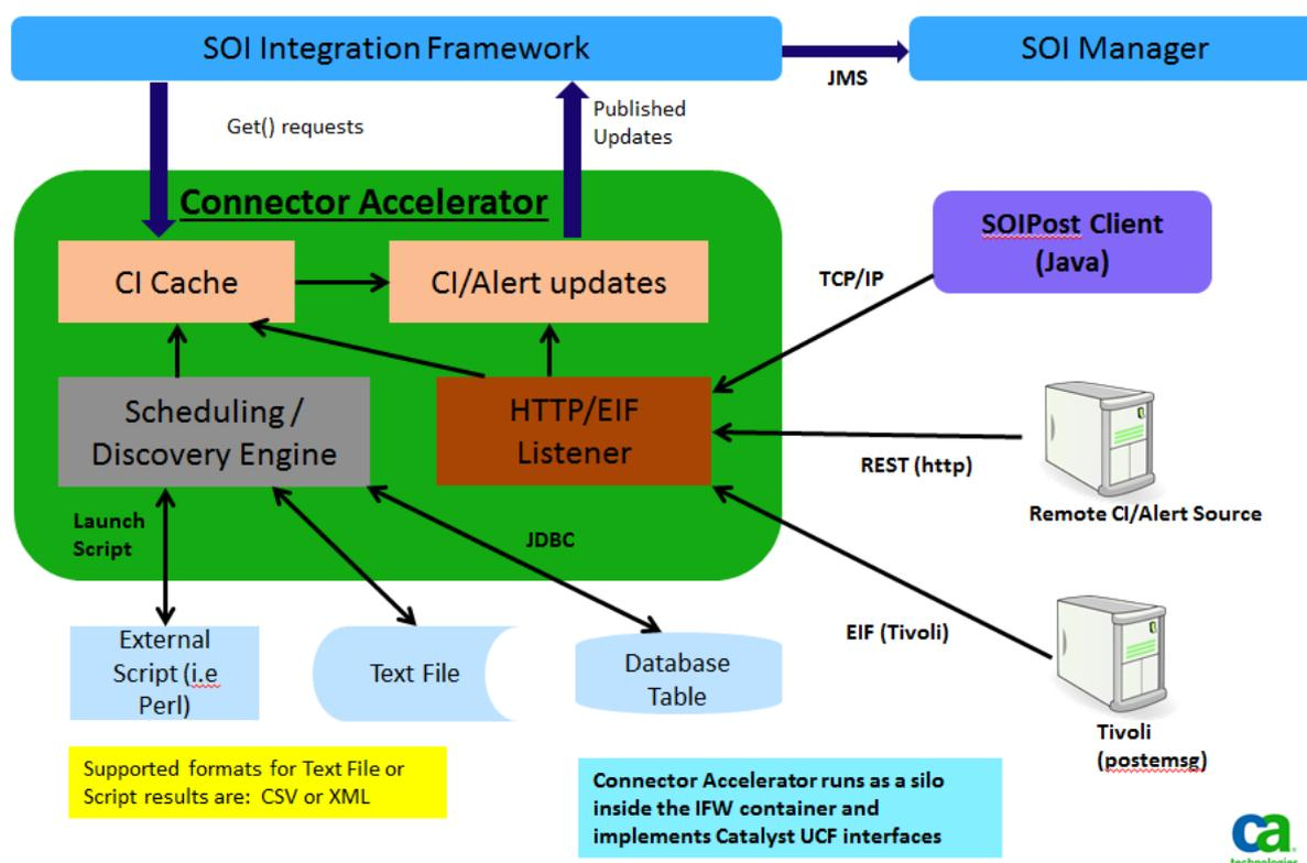
The Connector Accelerator contains the following primary components as outlined in the above diagram:
