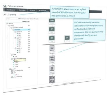
In CA Performance Management r3.0 and combined with CA Virtual Network Assurance r2.0, we introduce a new out of the box dashboard called "ACI Console" to provide a starting point for users to monitor Cisco ACI data center. The ACI Console allows the users to see a global view of the ACI data center covering physical, virtual and logical items and includes an innovative relationship topology of the interdependencies of these ACI items.
