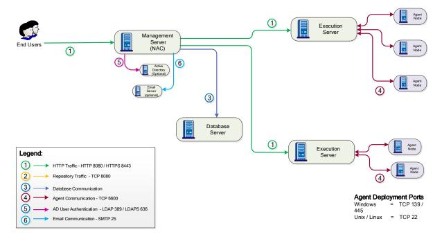
The schematic shows the various components that make up a typical CA Lisa Release Automation deployment.
