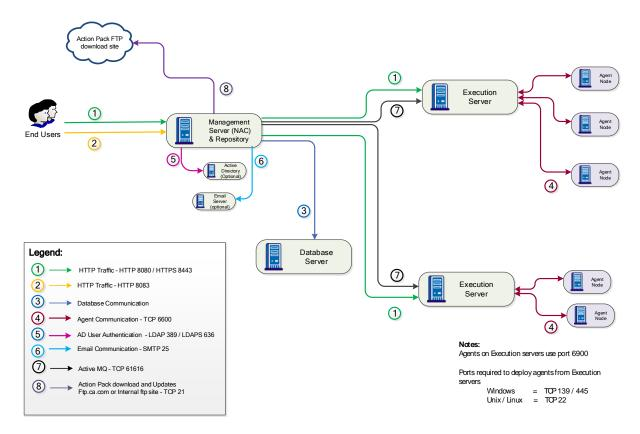
The schematic shows the various components that make up a typical CA Release Automation deployment.
