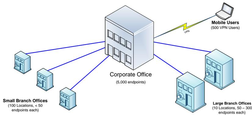
Multiple design scenarios are possible for large enterprises using a multi-tier reporting model. In most cases, this model includes a main campus, small and large remote locations, and itinerant users that connect across the WAN. The following graphic represents a multi-tiered approach for a large enterprise to manage resources and generate reports, providing regional and corporate management across the WAN and local management across the LAN.
