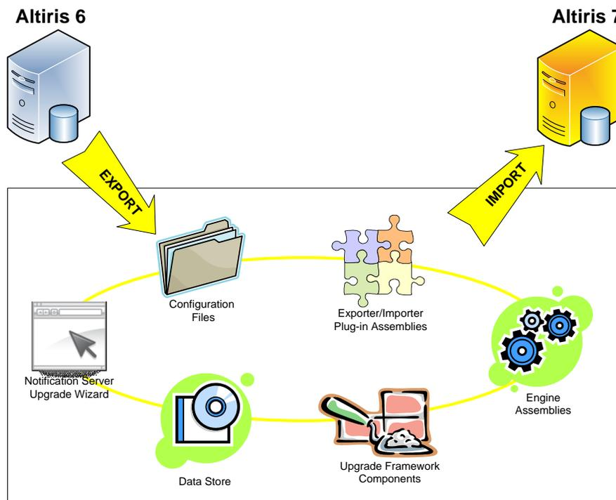
The migration process in Altiris 7 has been redesigned to give you more control. For example, you can now specify the location of the installation files and a data store, which stores data files from the Client Management Suite 6.0 database. The Specific elements and processes are described below:
