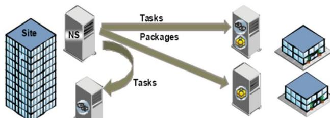
Altiris Site Servers with the Package Services option enabled act as local file servers for devices that have the Altiris Agent installed. A package is defined as a collection of files, scripts or a command line that is created by Software Management Solution that must be delivered from the Notification Server to the client. When the administrators enable packages on the Notification Server, the packages are replicated to all of the Site Servers that are known by that Notification Server.
