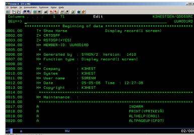
The "RPG Program" Loads the DDS via the definition as an externally described file. Assigns the variables and writes to 5250
